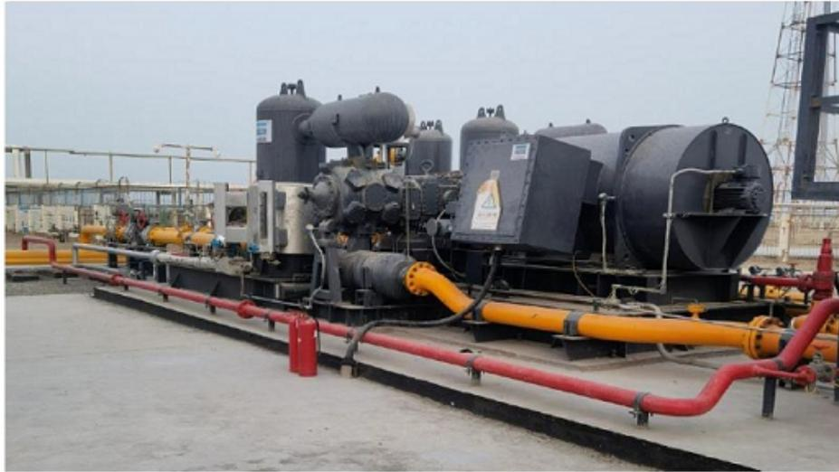
*Our high-pressure and ultra-high-pressure gas injection compressor units.*
