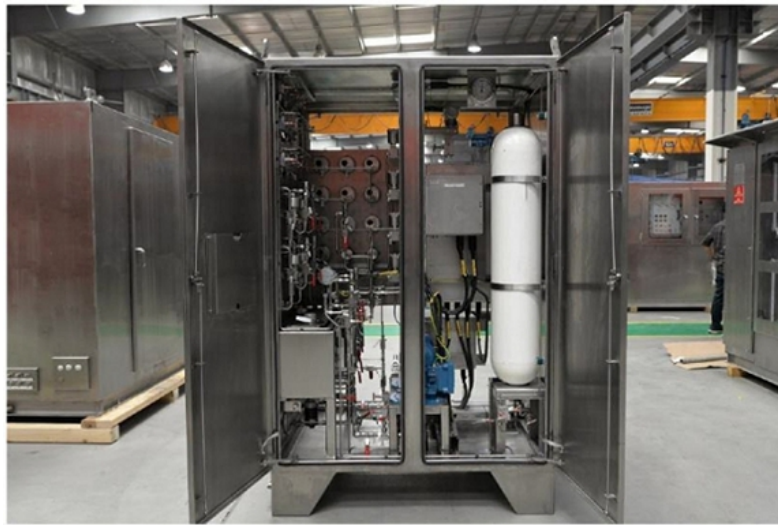
Our wellhead safety control system.
