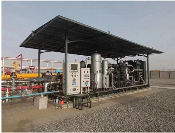
Our single-well or multi-well natural gas booster compressor units and downhole gas lift nitrogen production integrated compressor units.
