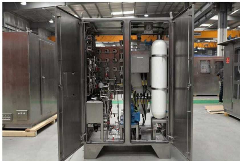
Our wellhead safety control system.
