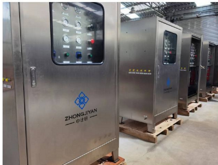
Our wellhead safety control system.
