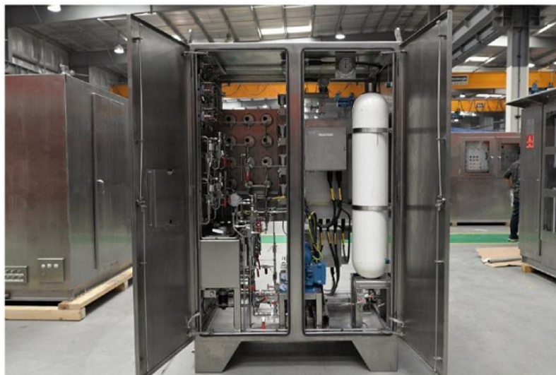
Our wellhead safety control system.
