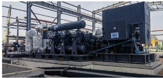
Our ultra-high pressure gas injection compressor unit.
