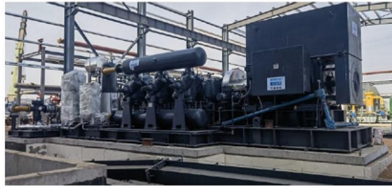
Our ultra-high pressure gas injection compressor unit.
